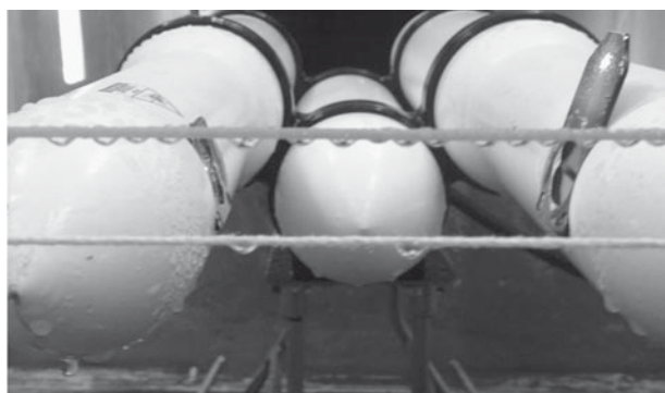
Fig. 4. Illustration of saturation and droplet accumulation on nylon (upper) and cotton (lower) strings
