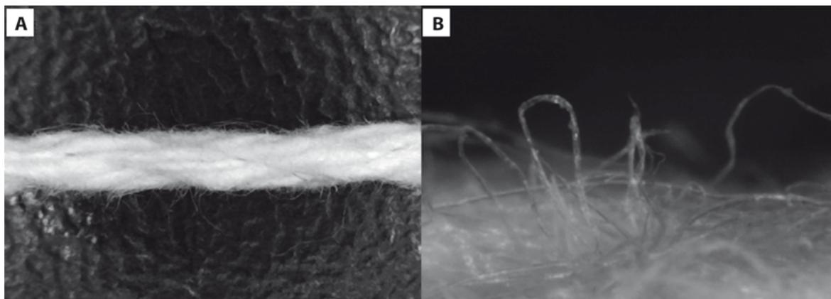
**Fig. 3.** A – 20 $\times$  view of the cotton string illustrating physical differences in diameter as well as the fibrous nature of the textile, B – a 400 $\times$  view of the outstretched fibers, approximately  $15 \text{ } \mu\text{m}$  thick
