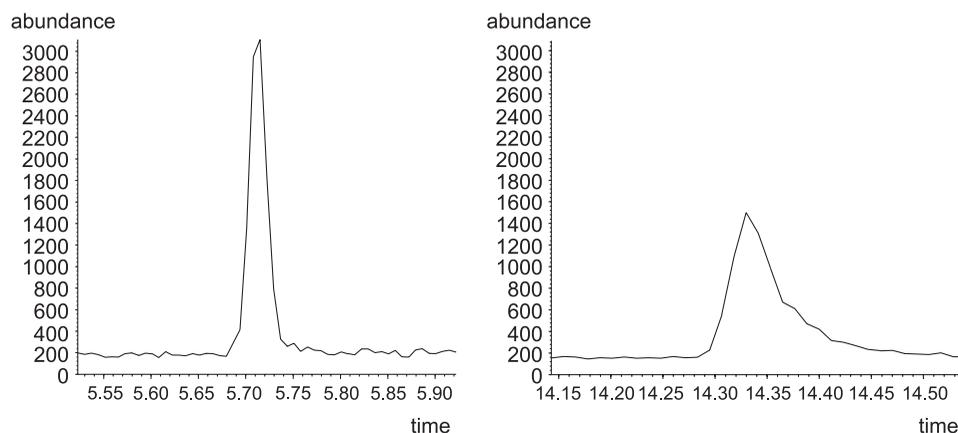
Fig. 1. Peak-shapes of chlorothalonil obtained by LP-GC/MS and GC/MS
