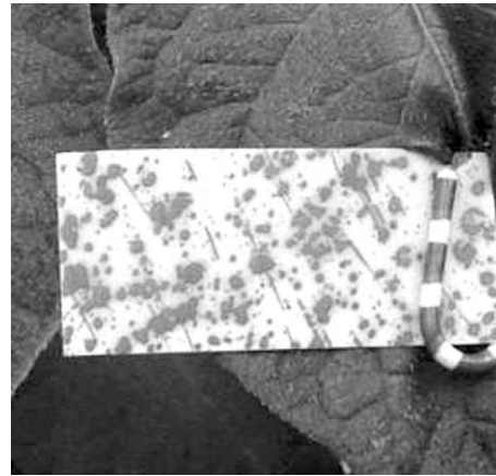
Fig. 1. The method of placing water sensitive paper on leaves
