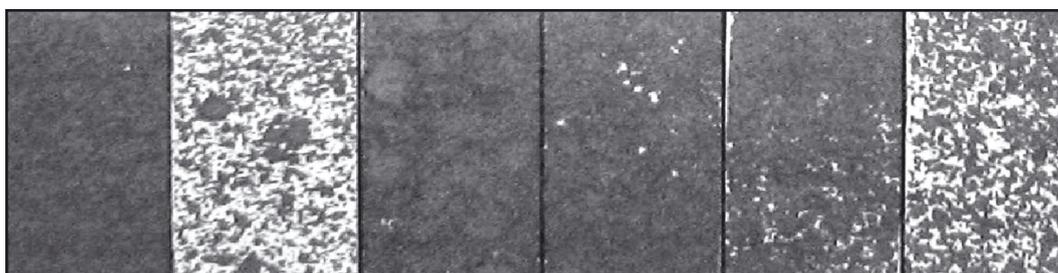
Fig. 1. Distribution pattern of spray spots on water sensitive papers
