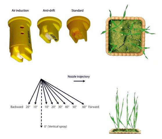
**Fig. 1.** Wild barley having vertically-oriented leaves at herbicide application time, the nozzles used in the study, and the angling of their spray from 20° backward to 60° forward relative to the direction of nozzle trajectory
