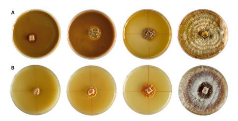
**Fig. 4.** Antifungal effects of (A) binary compound AgCl + ZnO and (B) single compound ZnO tested at different concentrations against *Cryphonectria parasitica* added directly into the cultivation medium, *in vitro* growth inhibition test on Petri dishes left to right: (A) different concentrations of reagent 0.25 g, 0.125 g and 0.05 g  $\cdot$  100 ml<sup>-1</sup>, negative control, (B) 0.2 g, 0.1 g, 0.04 g and 0.01 g  $\cdot$  100 ml<sup>-1</sup>
