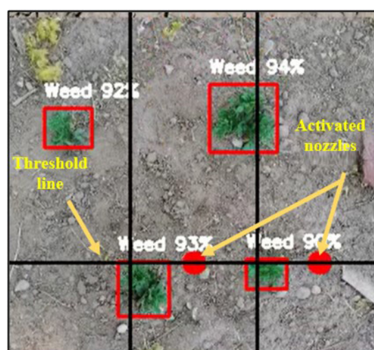
Fig. 3. Shows the threshold line and how the nozzles (illustrated in red circles) is work when detecting artificial weeds
