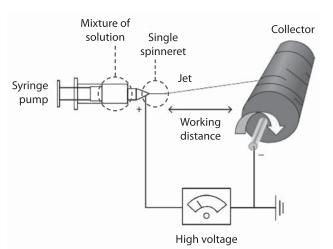
**Fig. 1.** Schematic diagram of the eletrospinning setup (Mori *et al.* 2015)
